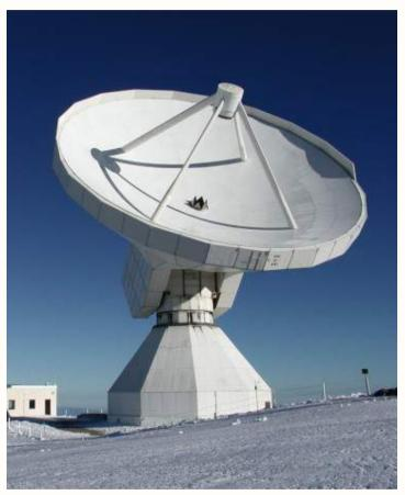
$\nu \sim 217.3$  and 233.0 GHz Angular resolution  $\sim 12$ " ( $\sim 0.5$  pc) Spectral resolution: 0.3 kms<sup>-1</sup> Line observations
