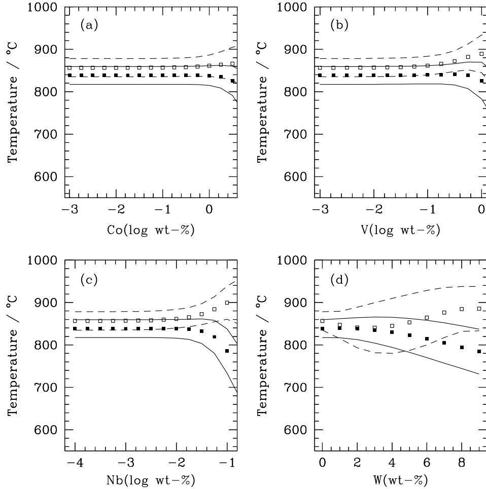
Figure 6: Gaussian process model predictions for Co, V, Nb and W. The filled points are the  $Ac_1$  predictions, and the solid lines the corresponding  $\pm 1\sigma$  modelling uncertainties. The open points are the  $Ac_3$  predictions, and the dashed lines the corresponding  $\pm 1\sigma$  modelling uncertainties. The alloys are Fe–0.2C (wt-%) steels; the heating rate is  $1 \text{ K s}^{-1}$ .
