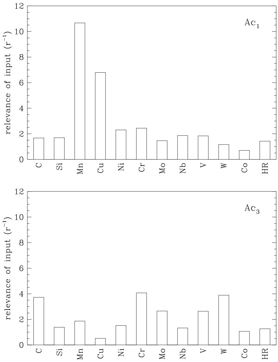
Figure 3: Model inferred relevance of the 12 inputs for the  $Ac_1$  and  $Ac_3$  Gaussian process models. HR is the heating rate. The relevances are the inverses of the length scales,  $r_l$ .
