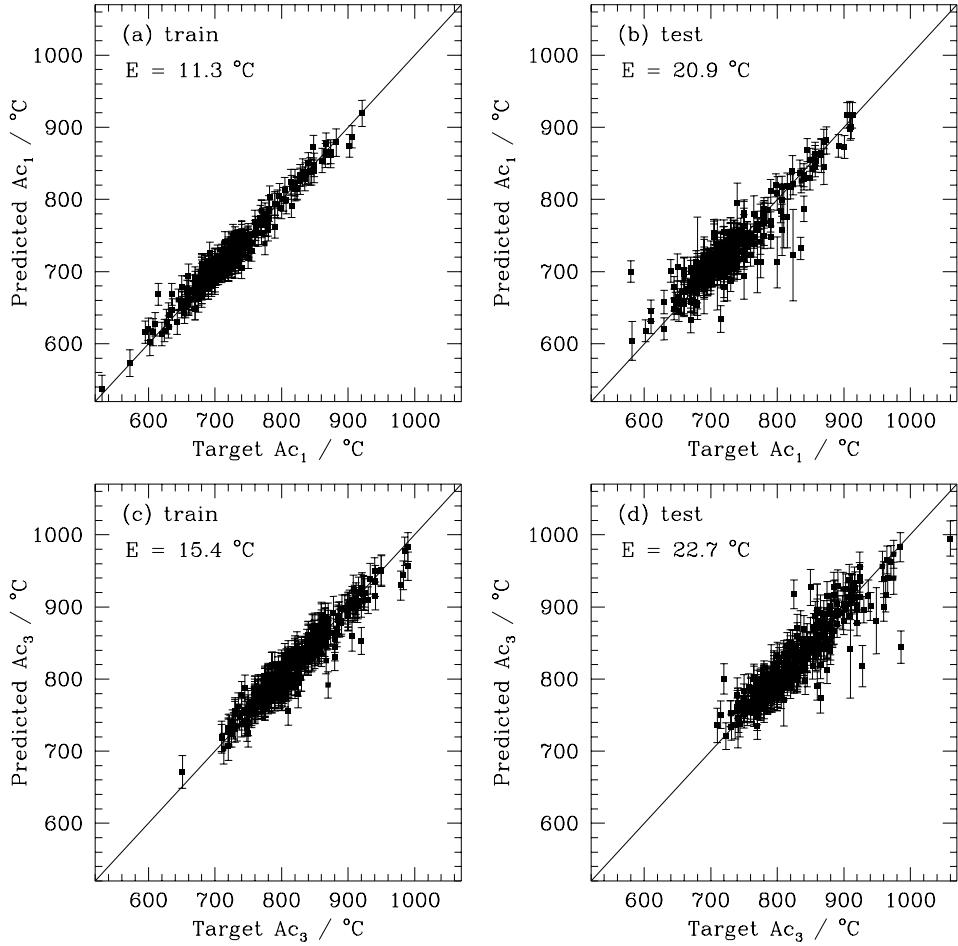
(a)  $Ac_1$  model predictions of the training data; (b)  $Ac_1$  model predictions of the test data; (c)  $Ac_3$  model predictions of the training data; (d)  $Ac_3$  model predictions of the test data.
