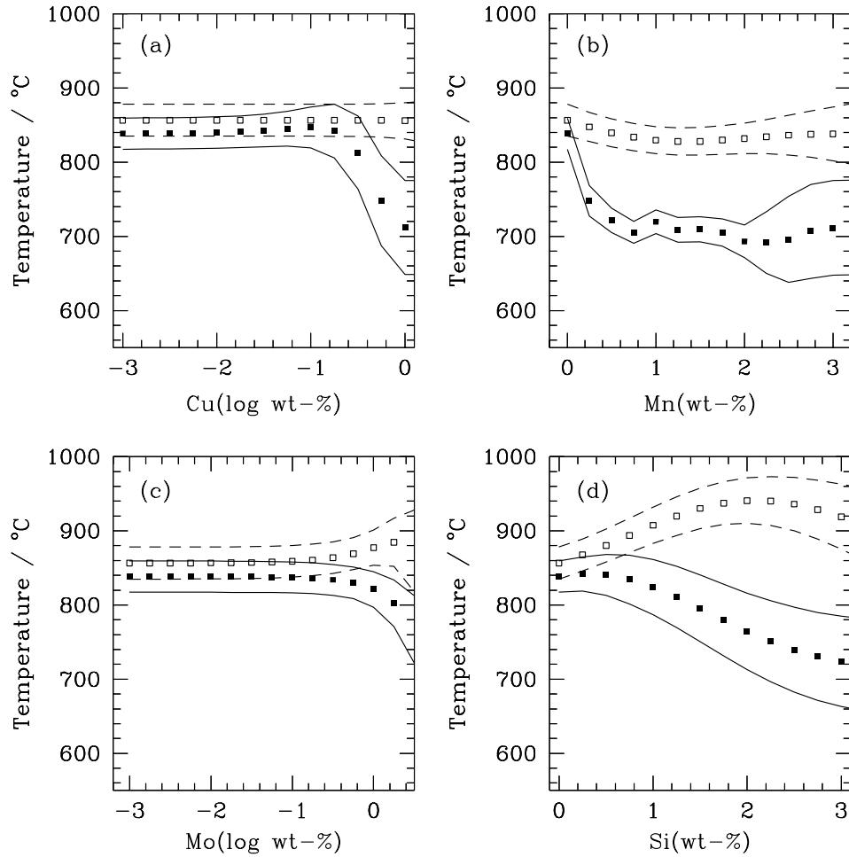
Figure 5: Gaussian process model predictions for Cu, Mn, Mo and Si. The filled points are the  $Ac_1$  predictions, and the solid lines the corresponding  $\pm 1\sigma$  modelling uncertainties. The open points are the  $Ac_3$  predictions, and the dashed lines the corresponding  $\pm 1\sigma$  modelling uncertainties. The alloys are Fe–0.2C (wt-%) steels; the heating rate is  $1 \text{ K s}^{-1}$
