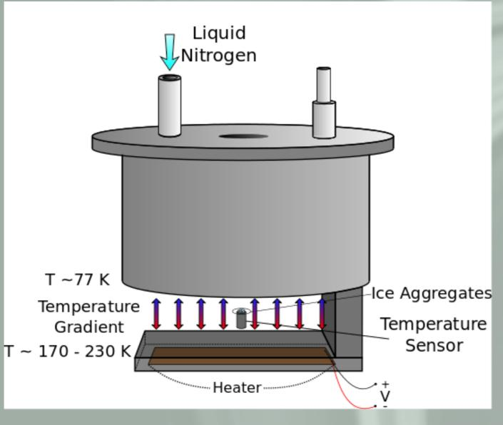
Water ice agregates are formed by hit and stick processes and aggregation in a cooled vacuum chamber. The top part of the chamber is covered by a liquid nitrogen container and a heater is situaded at 4 cm below to create a temperature gradien. A temperature sensor, used as target, is situated between the lower part of the container and the heater. The aggregates formed on the sensor are observed with a high speed camera for later study.
