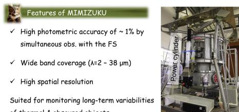
Fig. 3. Fabricated dewar of MIMIZUKU (2-m cubic, 2.3-ton). Details are described on <http://www.ioa.s.u-tokyo.ac.jp/TAO/mimizuku/pub/>. 'MIMIZUKU' means 'owl with long ears' in Japanese.
