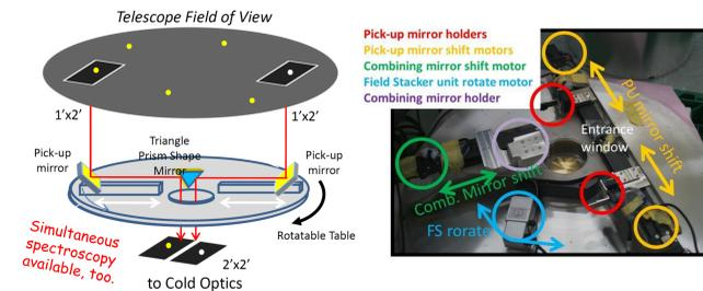
Fig. 4. (left) Schematic view of the FS. (right) FS components around the entrance window of the dewar. These motions enable free field pick-up. Two power cylinders are attached to the sides of the dewar as shown in Fig. 3. They move the dewar up-and-down to cancel out variation of optical path-length caused by PU-mirror shifts.
