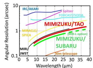
Fig. 7. Comparison of angular resolution between the MIMIZUKU and recent/future MIR instruments.
