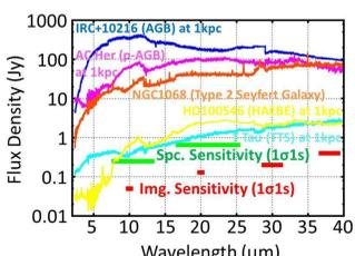
Fig. 8. Estimated sensitivity of the MIMIZUKU and some scaled spectra of interesting objects
