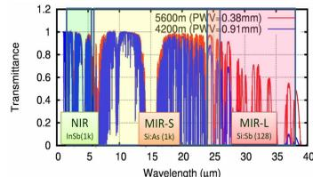
Fig. 6. Atmospheric transmittance and band coverage of the MIMIZUKU.
