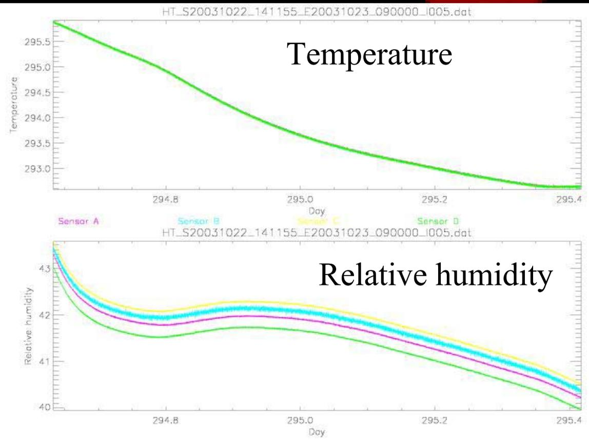
Four sensors have been positioned in a box. Temperature and humidity readings for all 4 sensors are presented below for a test environment at Leiden. Note that the four temperature readings fall on top of each other. For humidity there is a small spread, a consistent off-set between the four sensors. The drop in temperature is due to cooling over night. The graph starts at 2 pm until 10 am the next day
