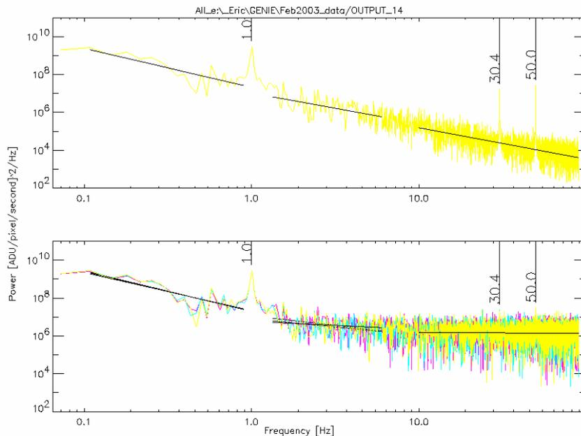
The simulated data is build on one of the real datasets (time sampling). 1 Hz, 30 Hz and 50 Hz sinus signals have been added for the MIDI closed cycle cooler (1 Hz), and the power line frequency (50 Hz), and one for a yet unknown source (30 Hz).
