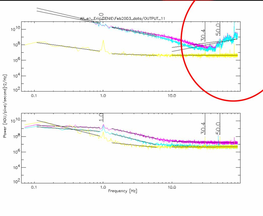
During experiment exp11, engineers were working at UT3 to fix technical problems with the Coude optics. This has apparently introduced significant power above 50 Hz, and an overall increase of the power for low frequencies (0 to 10 Hz).
