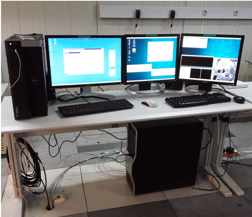
Figure 4. A view inside the old NTT local control room: the Astralux Sur remote camera computer pleione2 on the table left, and the pipeline computer apipe2 below the table. The image shows the orange fiber cable on the left and the white 8-port network switch on the very right of the table.
