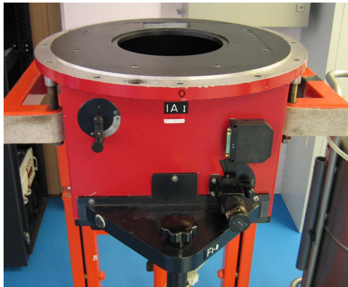
Figure 3.19. The Instrumentenansatz 1. The filter wheel FI-8 is mounted in the lower part of the IA 1 and can be rotated either remote or manually via the black knob on its top.
