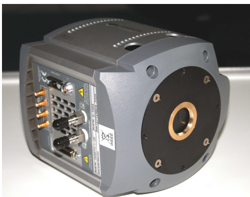
Figure 3.2. The AstraLux DV887-UVB camera head. The connectors for optional water cooling, external triggering, power supply and data transfer are visible on the left side of the camera housing.
